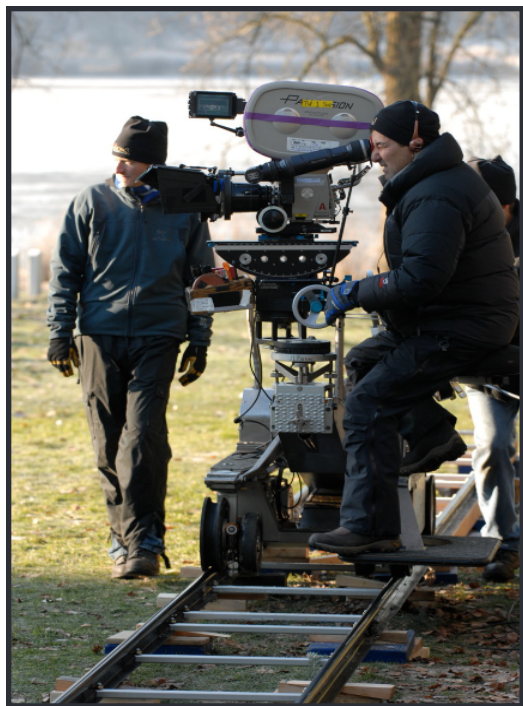
Standard dolly package track setups require minimal support cribbing every 4' at joins and midsections resulting in faster setup time.
