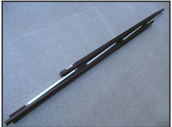
Scissored 8' section for storage. ( 10' L x 6" W x 3" H and weighs 40 lb.)
