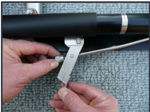
Knurled nut tension adjuster on latch for connecting track sections together.
