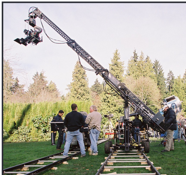
Track can be customized for various widths to accommodate both dolly and crane configurations. Maximum load 6500lbs. when supported every 2 feet.
